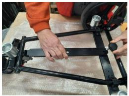
Rotate the handle upwards and by acting on the red knob lock it in the desired inclination. Screw the two locking knobs of the vertical structure. Position the ballast with 5/6 kg of stones or sand inside (not supplied)
