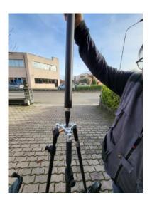
Loosen the locking knobs of the tripod's extensible legs and by acting on the buttons, level the pole, lock the pole and close the leg locking knobs
