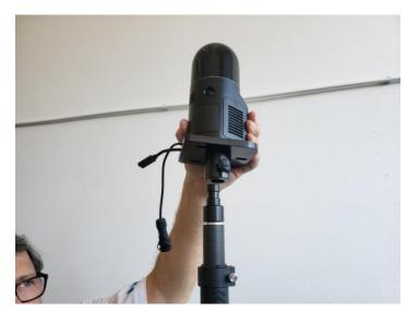
Lock the instrument by screwing the side knob, open the connector cap
