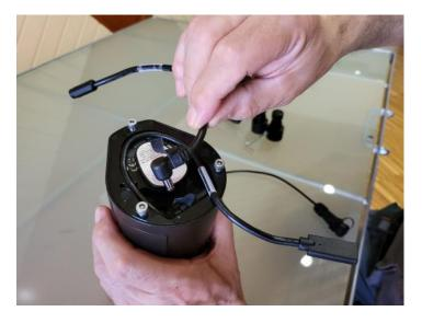
Do not wrap the cable around the bottom of the scanner
