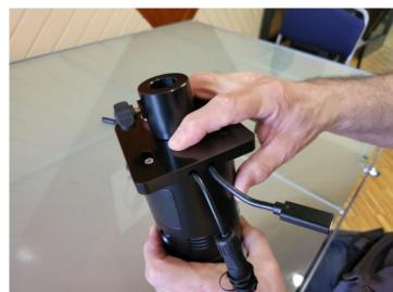
Place the bracket on the locking screws and slide it to the fixation position
