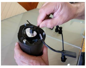
Mount the bracket by letting the cables enter into the appropriate seats
