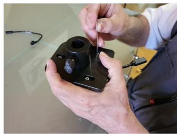
Screw the 5/8" female adapter on the carbon pole and mount the instrument
